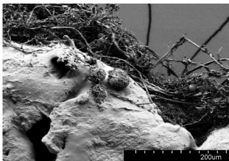
pics by scanning electron microscope 4) SEM, Lichen inside GROWLAY (Flechte)
