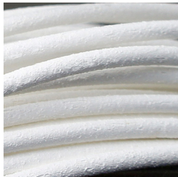
DI-ELECTRO-LAY , filled with TiO 2 72%
