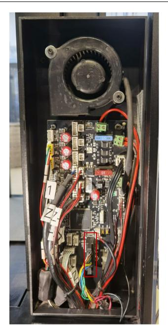
6. Disconnect the extruder signal cable from the motion controller board, connect it to the gray connector of the extruder signal adapter cable, and close the gray connector buckle so that the black connector of the extruder signal cable can be fixed to the gray connector buckle. The finished result is outlined in red in the following image.
