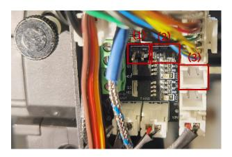
4. Connect the three connectors of the auto-leveling assembly respectively to the three terminal blocks shown in Step 3. As outlined in red below, connect the brown wire to the 2-pin terminal block (1), the white wire to the 3-pin terminal block (2), and the red and black wires to the white terminal block (3).
