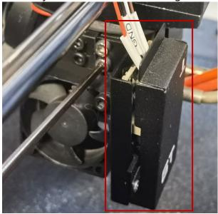
3. Locate the extruder board on the upper part of the extruder, as well as the three unconnected terminal blocks on the extruder board (fig. (1), (2), and (3) below).
