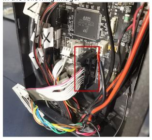
8. Connect the small white connector of the extruder signal adapter cable to the terminal J32 on the motion controller board, as outlined in red in the following image. Finally, close the electronic box cover. The installation of the auto-leveling assembly upgrade kit has been complete.
