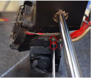
2. Thread the two screws removed in Step 1 through the screw holes on the auto-leveling assembly and reinstall them onto its original position. Tighten the screws. The auto-leveling assembly will be fixed next to the right fan, as outlined in red below.
