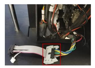
7. Connect the black connector of the extruder signal adapter cable to the terminal block where the extruder signal cable was plugged in Step 5. The finished result is outlined in red in the following image.
