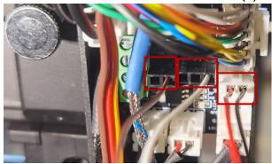
5. Open the side door of the printer, and then open the electronic box cover at the bottom of the printer to expose the motion controller board inside the electronic box. Locate the extruder signal cable on the motion controller board, as outlined in red in the following image.
