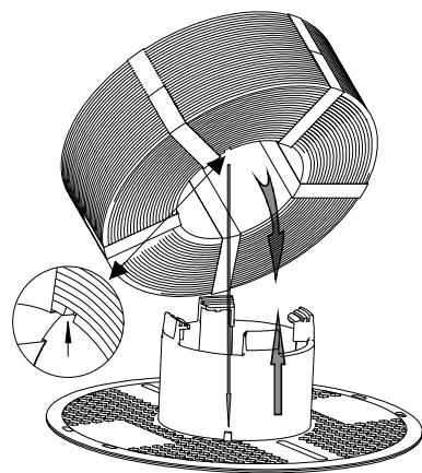
3.1 □ Press the detached part of spool and rotate it clockwise until it is assembled in place
